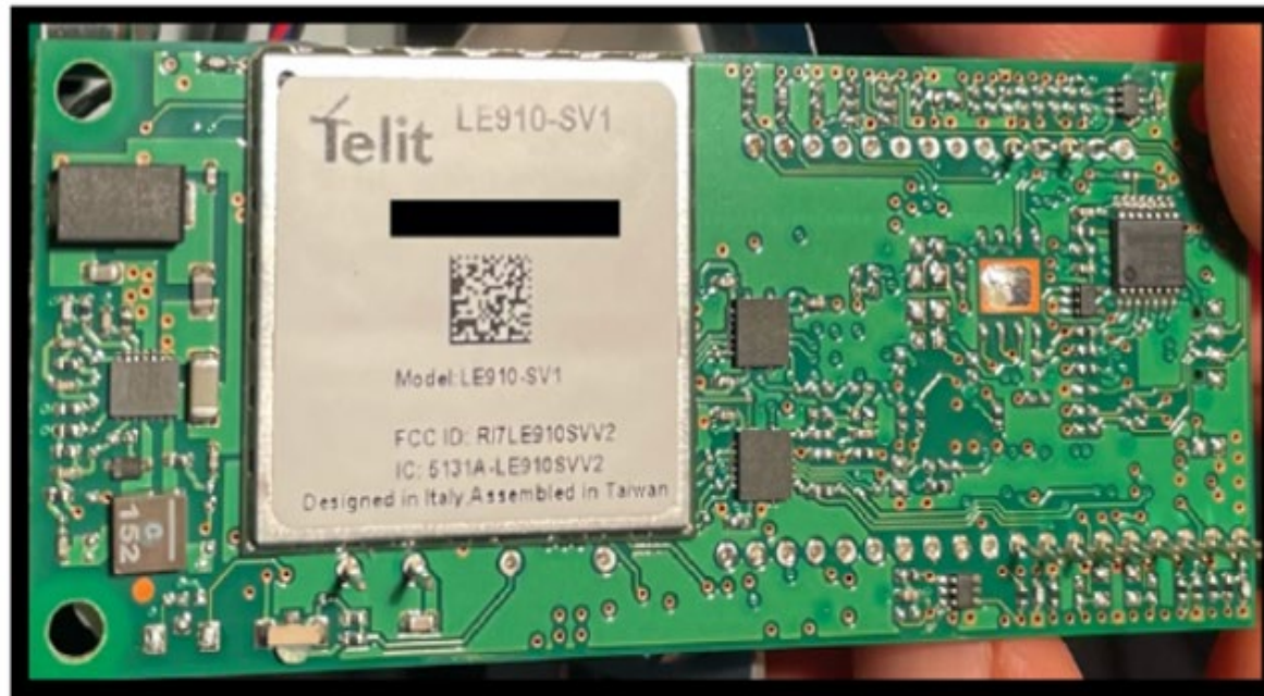
ESS DS200 Motherboard with Telit LE910-SV1 Modem Chip
